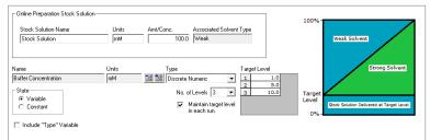
Maintain target level in each run: the software can maintain the target OLP variable in a given run (injection) as an absolute constant within the mobile phase independent of the change in the Strong/Weak solvent ratio across the gradient.
