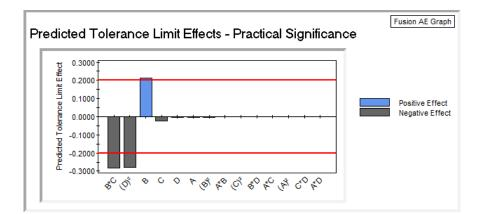
Maximum Allowable Difference from Mean: |Predicted Tolerance Limit Effect| < 0.2 for each variable studied.
