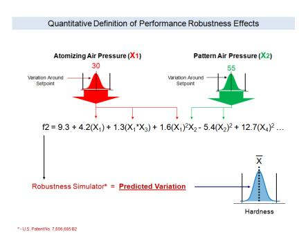
**Fusion Pro** equations derived from the experiment data characterize the effects of the experiment variables on each analyzed response (CQA). **Fusion Pro** can combine these equations with the Monte Carlo Simulation equations for predicting robustness into its global Best Answer Search utility to find the best overall conditions from the current experiment.
